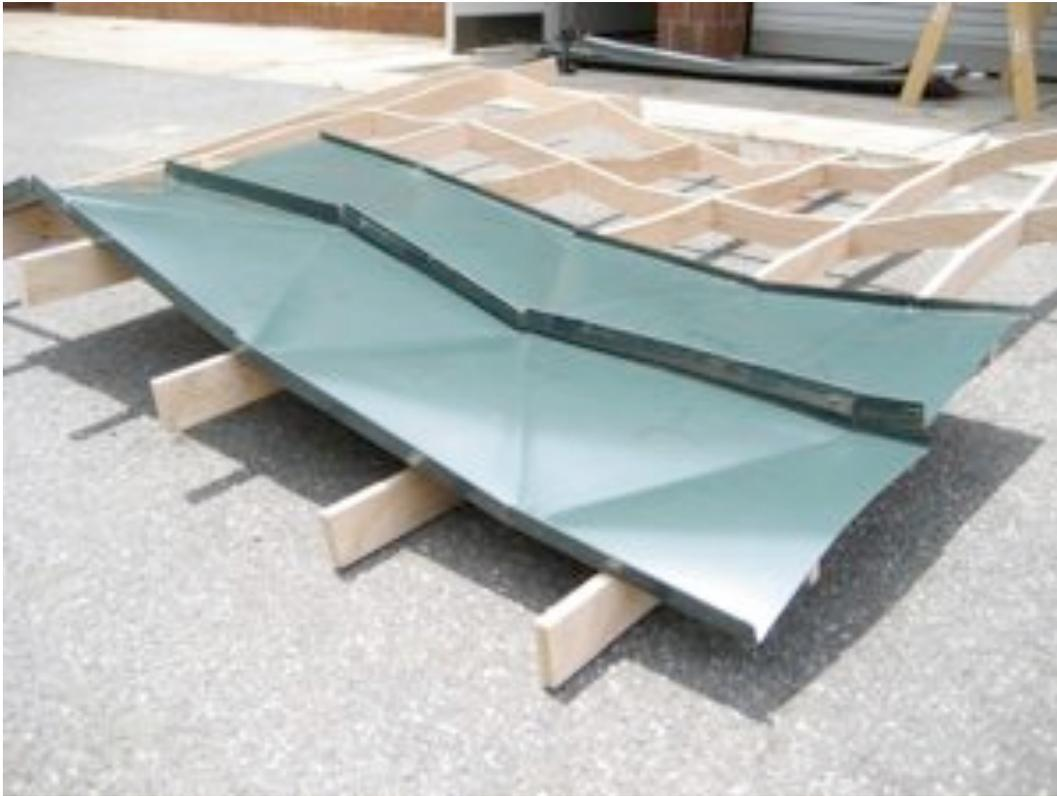
**Figure 6-** Standing seam test on frame
