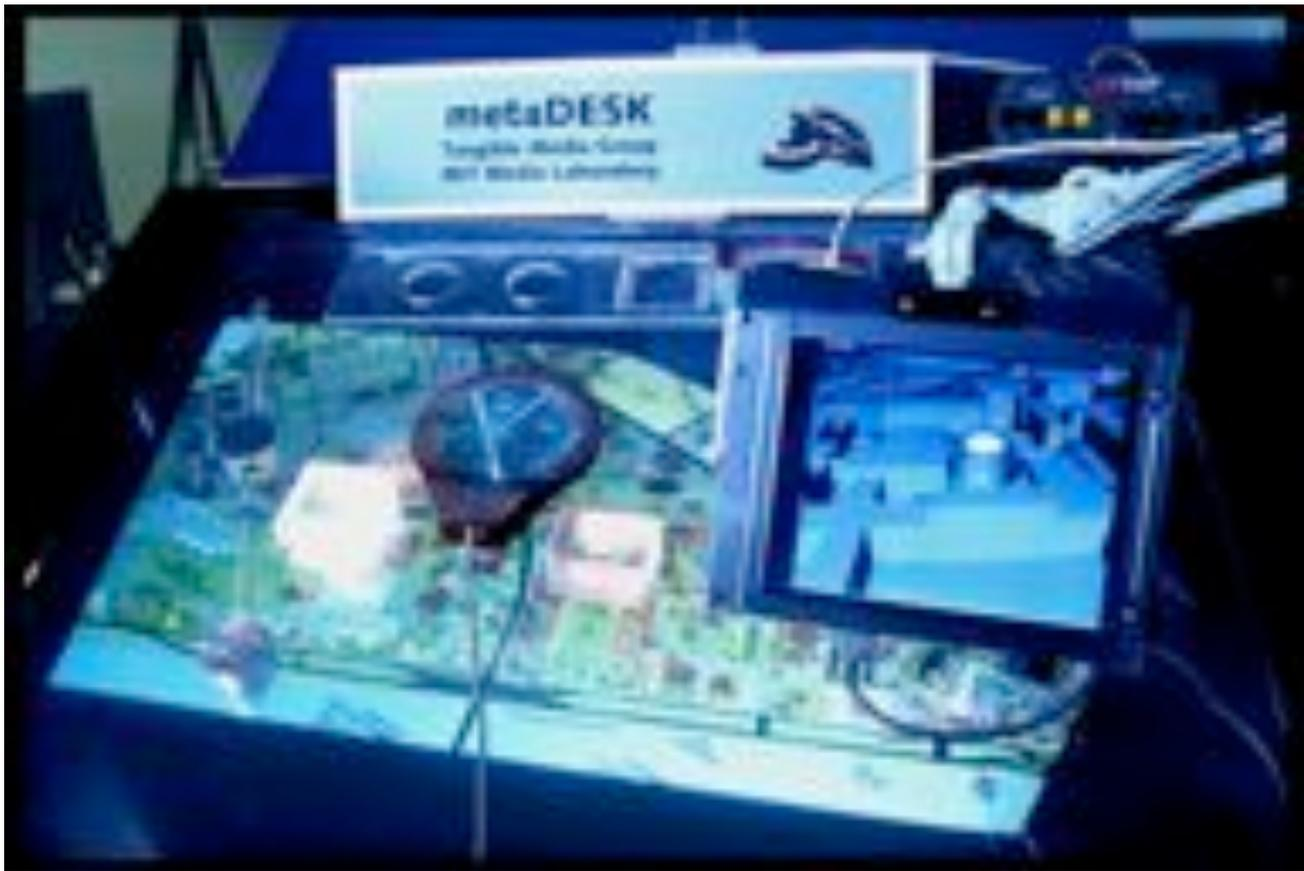
**Figure 1: metaDESK, designed by the Tangible Bits Research Group at MIT's Media Lab**
